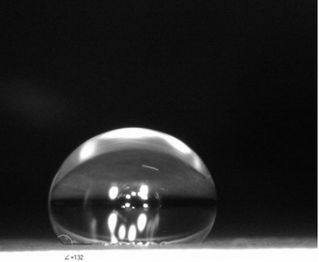
Fig. 4. Contact angle of water drop on aluminum surfaces. (a) coated Al. (b) coated anodize Al.
