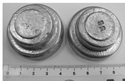
Fig. 1. Samples for testing the alloy porosity content
